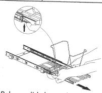
2. Release slide by pushing the black trigger UP on the LEFT side and DOWN on the RIGHT side
