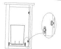
Make sure the cabinet hinge will not interfere with organizer when installed
